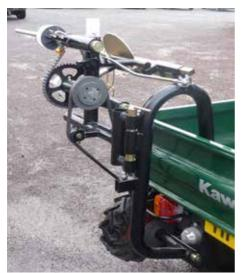
The belt position is crossed in a figure of eight between the Top Pulley and Wheel Arm Pulley.
