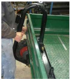
When the frame is in place mark the position of the mounting frame holes in the bed. Check underneath for wires, pipes and clearance. You can now drill and bolt through the bed and secure the mounting frame using the plates provided.
