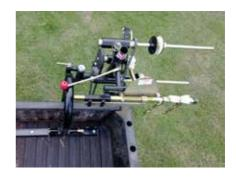
Slip the drive belt over Top Pulley and Wheel Arm Pulley twisting it to form a figure of eight.
