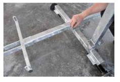
4. Join the Chassis to the Axle using bolts A x4.
