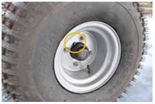
Replace the wheel nuts and tighten.
