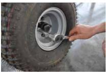
Place the Wheel (6) onto the Wheel Stub (2). The wheel rim must line up with the grease nipple (located on the Wheel stub) in order to fit correctly.
