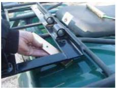
4. Attach the winder to the wheel arm using the connection pin ensuring the reel shaft is on top of the machine. Swing into working position. Rotate the winder fully to check that there is clearance on all moving parts between the winder and the AT\/
