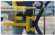
Tighten the clamp plate bolts. It may be necessary to trim the ATV mudguard and adjust the position of the rear lights if fitted
