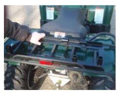
2. Attach the wheel arm to the mounting frame with the large pin. The wheel should sit on the offside rear tyre. Move the arm until the drive wheel is just outside of centre of the ATV tyre and the connection tube for the winder is close to vertical. tipping slightly towards the bike.
