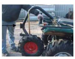
1. Place the mounting frame to the 3. Once the required position is reached, secure the mounting frame with the clamping plates and lightly tighten. Try to clamp the mounting frame onto the strongest part of the rack.
