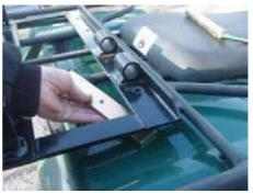
4. Attach the winder to the wheel arm using the connection pin ensuring the reel shaft is on top of the machine. Swing into working position. Rotate the winder fully to check that there is clearance on all moving parts between the winder and the ATV.
