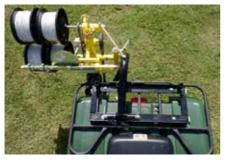
Push the winder towards the bike and slip the drive belt over the Top Pulley and Wheel Arm Pulley twisting it to form a figure of eight.
