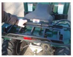
Attach the wheel arm to the mounting frame with the large pin. The wheel should sit on the offside rear tyre. Move the arm until the drive wheel is just outside of centre of the ATV tyre and the connection tube for the winder is close to vertical, tipping slightly towards the bike.
