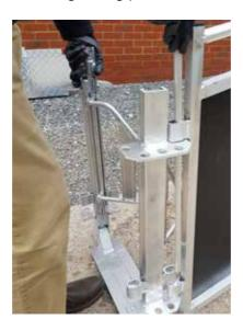
8. Fit the Entry Ramp (8). Secure by locating the pins to the Yard Attachment Bracket and locking with a Pipe Pin (3).
