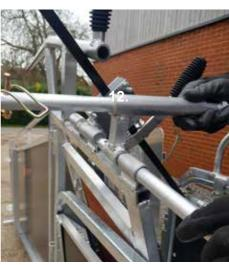
12. Pull the Panel Connector towards the Small Grip -Panel and secure using a Pipe Pin (3). Next Secure the Black Slider located on the RaceGrip Handle to the Small Grip Panel usingPipe Pin (3).
