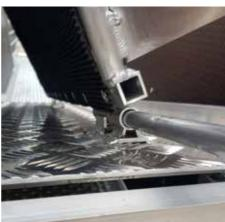
5. Place the Small Grip-Panel (5) onto the yard frame opposite the Large Grip-Panel. Secure using three Pipe Pins(3).
