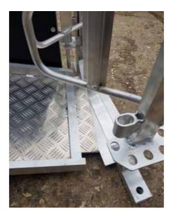
9. Position the short, Entry Panel -Left (9) opposite the long Entry Panel - Right. Locate the two round bars into the tubes on the platform. Secure to the Anti-Backing Gate with a long pin.
