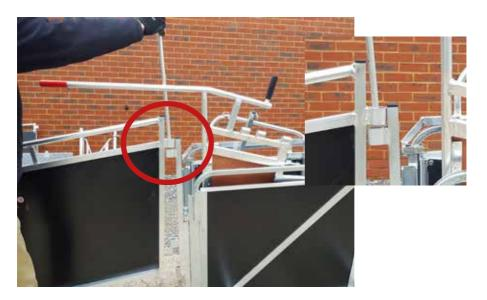
7. Place the Anti-Backing Gate (7) at the end of the entry panel. Secure to the panel using a long pin.
