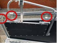
6. Place the longer, Entry Panel - Right (6) onto the Yard Attachment Bracket and secure with a long pin.
