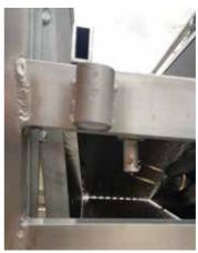
4. Remove the Long Pin from the Exit Ramp. Locate the Large Grip-Panel (4) and secure re-using the Long Pin.
