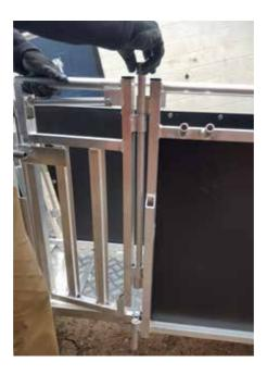
11. Locate the RaceGrip Handle (11) and the Panel Connector (12) onto the Large Grip - Panel and secure using a pin.
